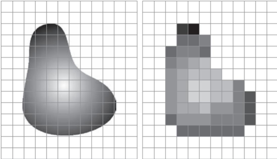
Figure 6: (a) Continuous image projected onto a sensor array. (b) Result of image sampling and quantization.
