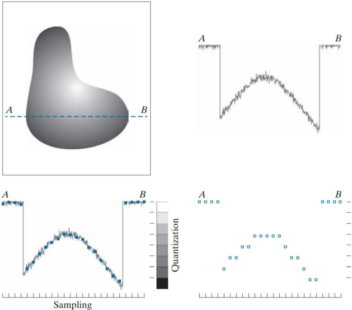
Figure 5: (a) Continuous image. (b) A scan line showing intensity variations along line AB in the continuous image. (c) Sampling and quantization. (d) Digital scan line. (The black border in (a) is included for clarity. It is not part of the image).
