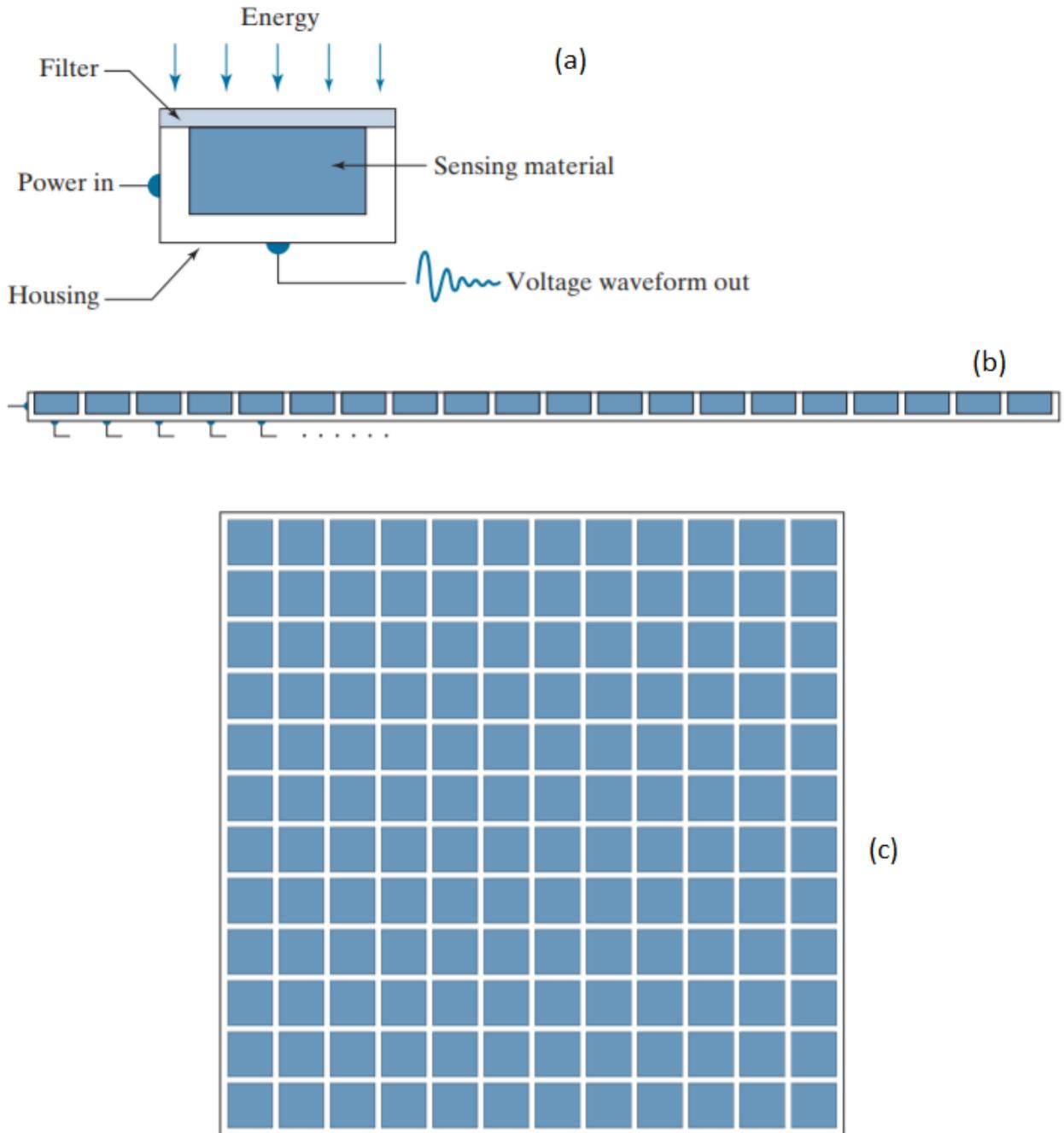
Figure 1: (a) Single sensing element. (b) Line sensor. (c) Array sensor.
