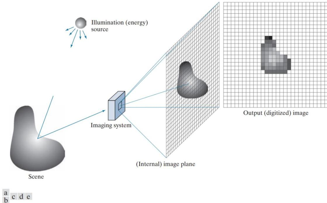
Figure 4: An example of digital image acquisition. (a) Illumination (energy) source. (b) A scene. (c) Imaging system. (d) Projection of the scene onto the image plane. (e) Digitized image.
