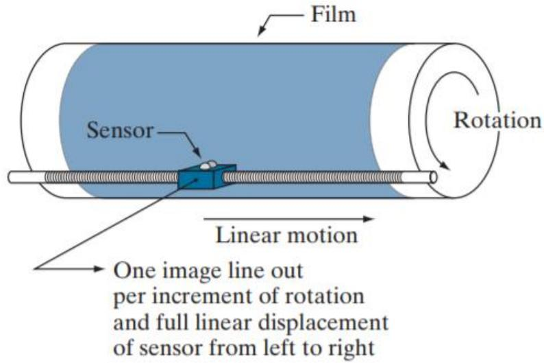
Figure 2: Combining a single sensing element with mechanical motion to generate a 2-D image.
