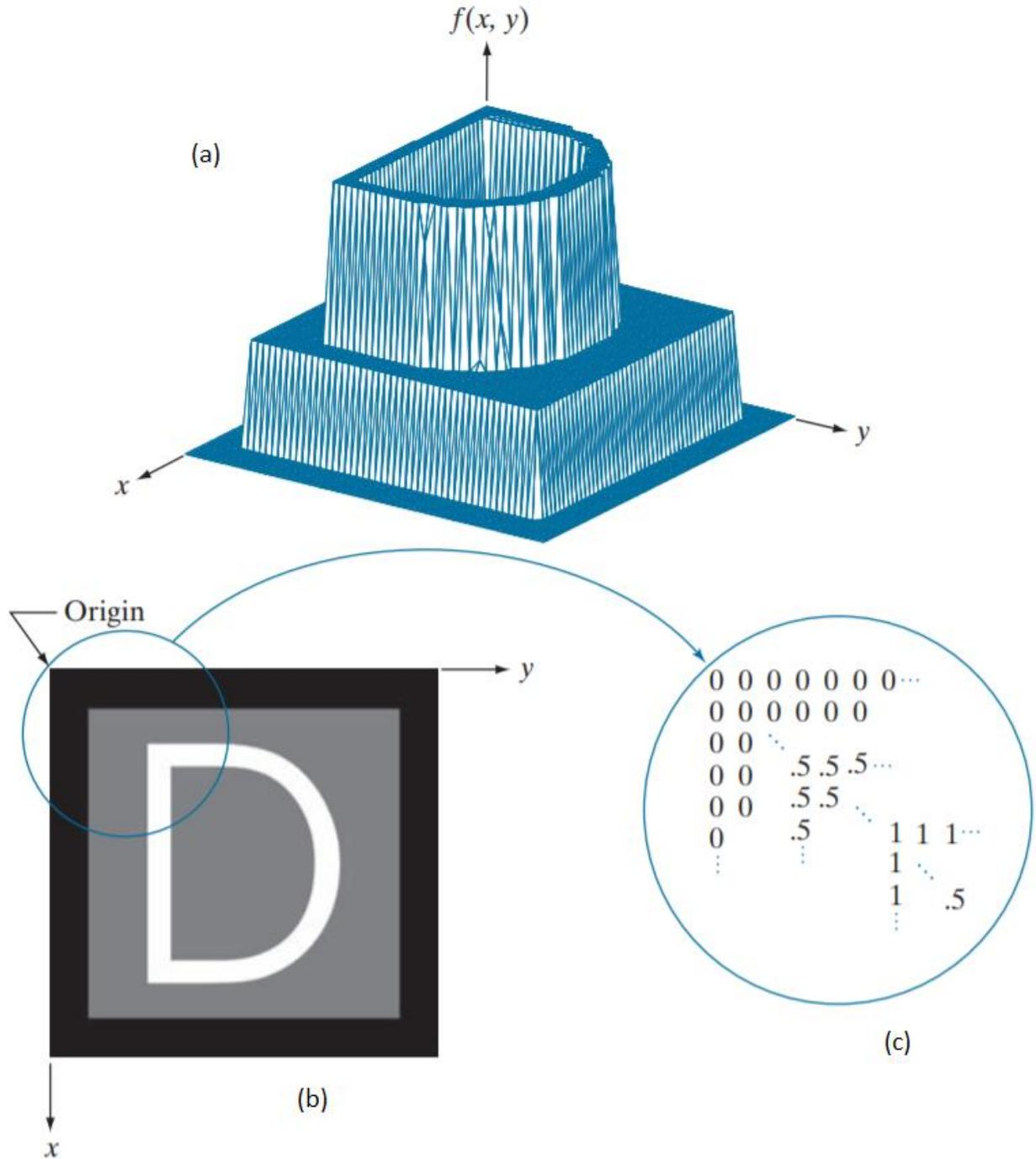
Figure 7: (a) Image plotted as a surface. (b) Image displayed as a visual intensity array. (c) Image shown as a 2-D numerical array. (The numbers 0, .5, and 1 represent black, gray, and white, respectively.)
