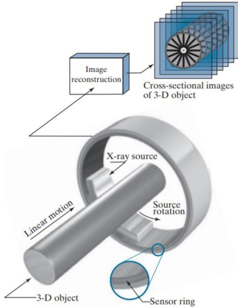
Figure 3: (a) Image acquisition using a linear sensor strip. (b) Image acquisition using a circular sensor strip.
